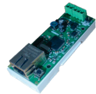
CNV1000 Converter RS485 to TCP/IP Does not require installation. IP address set through Internet Browser
